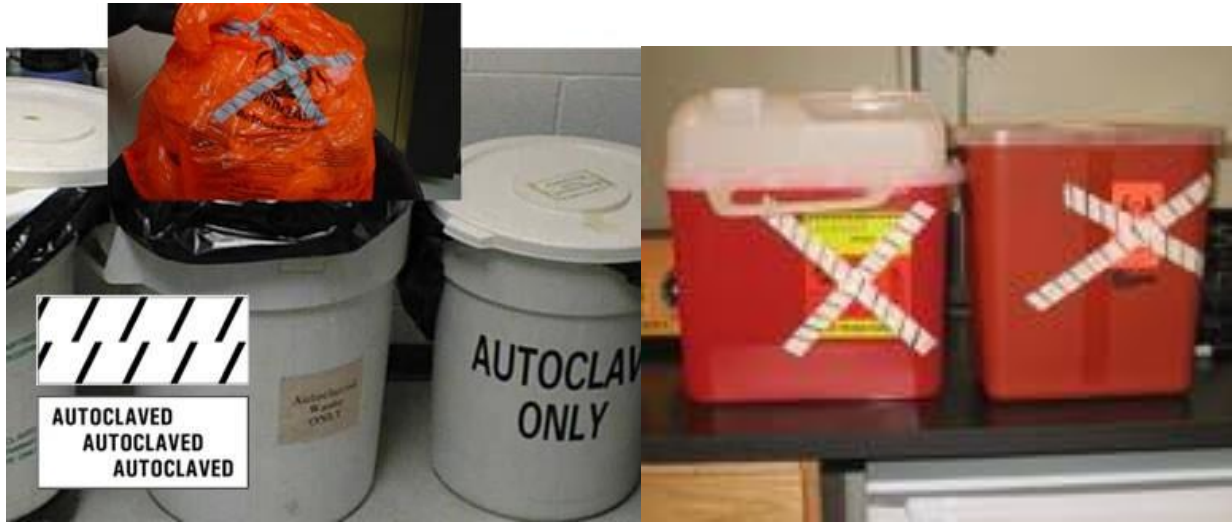
Figure 1 Autoclave tape utilizes a chemical reaction to indicate a temperature of greater than 121°C was achieved. This color change is usually displayed with hash marks or words that appear on the tape when proper temperature is reached.
