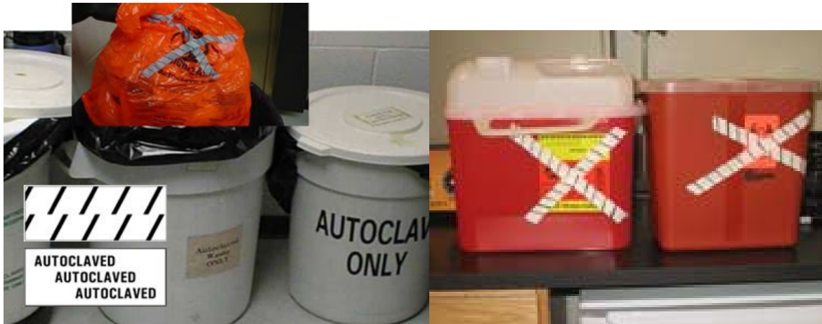
Figure 1 Autoclave tape utilizes a chemical reaction to indicate a temperature of greater than 121°C was achieved. This color change is usually displayed with hash marks or words that appear on the tape when proper temperature is reached.
